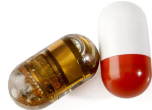
BodyCAP e-Celsius® ingestible biotelemetry capsule
